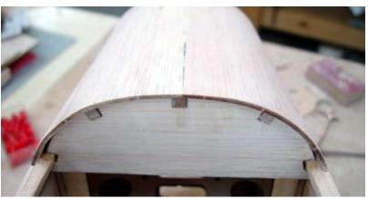
*The forward top sheet has been formed over the firewall at the front and F2 and the instrument panel in trhe cockpit area.*
