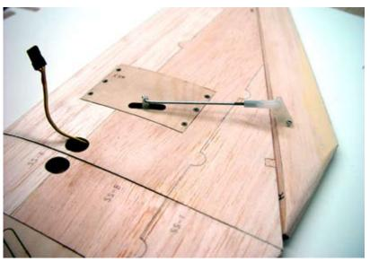
*The finished servo installation. Note that you will need a servo reversing Y-Connector to reverse one of the servos to get proper operation.*
