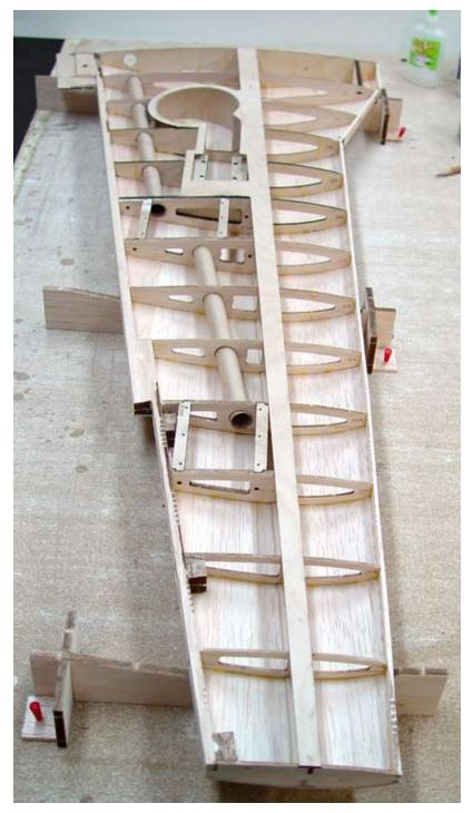
The left wing panel assembly nearing completion. The top sheeting has been installed and the assembly is placed in the bottom sheeting jigs. These jigs will support the wing and prevent any distortion of the wash out during the sheeting process. For all of it's complexity, at this stage it appears to be a relatively simple structure.
