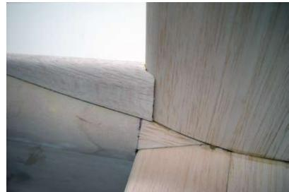
Installation of the vertical fin and dorsal fin. The dorsal fin is back sanded to form around the leading edge of the vertical fin.
