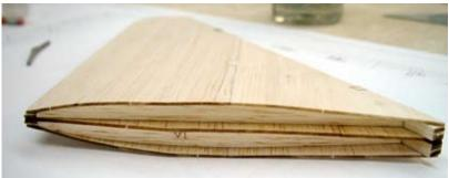
Assembly of the vertical fin completed and ready for final sanding and shaping of the leading edge. Very little additional shaping is required to form a perfect airfoil. Very light, very strong and very quick to build.
