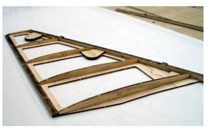
Assembly of the vertical fin underway with only one side completed. Note the core sheet splice on the right. The tabs on the trailing edge will position the sheeting when installed. The hinge pin openings have been capped with balsa and the assembly is ready to be turned over and completed.
