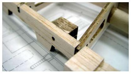
To provide more support for the aileron hinge points, these hinge blocks are added to the trailing edge of the aileron bay.
