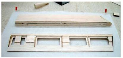
One aileron assembly completed and another ready for sheeting. The hinge caps and aileron horn plate filler have been installed and the all surfaces have been shaped to contour in preparation for sheeting.
