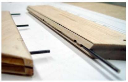
On the left is the vertical fin assembly with steel pins temporarily replacing the hinge pins and on the right is the rudder assembly. The double bevel on the rudder was cut using a band saw set at 35°. The rudder has been removed from the steel pins after marking the leading edge with the fin trailing edge. The rudder assembly can now be tapered to match the fin. The rudder torque rod is only temporarily installed and will be removed before finishing.
