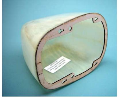
The cowl assembly ready to be customized for your model. The keyhole openings will engage shoulder head screws in the firewall to firmly retain the cowl. The 1/4" holes will contain magnets that along with the magnets installed into the firewall will prevent the cowl from detaching. To remove the cowl it must first be lifted and then pulled forward.
