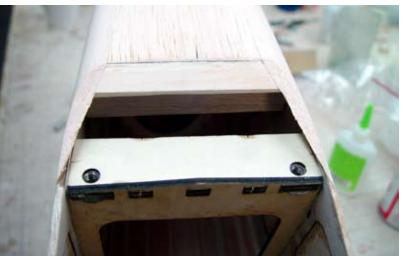
A piece os scrap balsa is used to fill in any remaining gap between the wing trailing edge and the fuselage wing opening.
