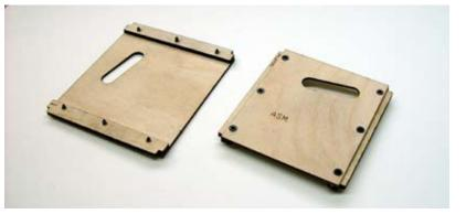
The flap and aileron mounts and their screw rails are temporarily assembled and then the rails are glued into there respective ribs. The servo mounts are then removed. This method assures perfect alignment of the components The flat head wood screws are countersunk to fit flush to the surface of the servo mounts. Note the materiel sticking out beyond the edges of the servo mount. This will provide a small shelf to support the wing sheeting.
