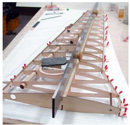
The top spar flange has been installed with Aliphatic Resin glue is curing under the weight of a straight edge to keep things laser straight. Note that the wheel well outliner is part of the spar flange and the lead weight is holding that down till cured.
