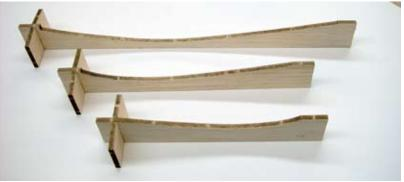
*RIGHT: The wing jigs for installing the bottom sheeting. They will support the wing assembly and prevent changes in wash out during the sheeting procedures.*
