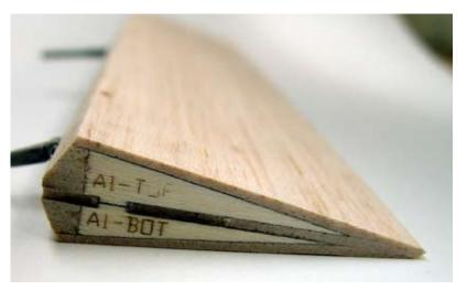
End view if completed aileron assembly showing the core sheet, leading edge, A-1 rib and sheeting. Very light and very strong.
