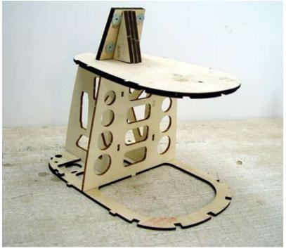
*This forward fuselage sub-assembly speeds the assembly. It consists of the firewall, F2, F2-A, F10, F8 and the nose gear mounting assembly.*
