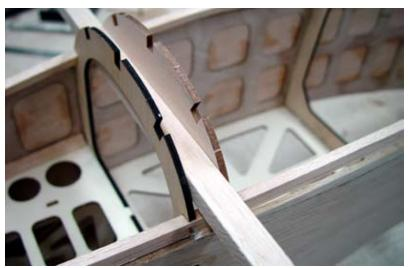
A piece of 1/2" scrap balsa is used to space the instrument panel 1/2" away from F2.
