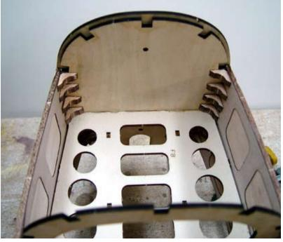
Bracing for the firewall is supplied by gussets both above and below F8.
