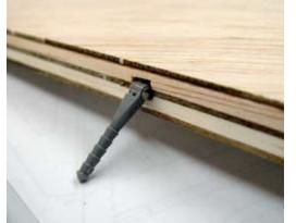
When the hinge pins are bottomed in the hinge pin holes, they are in the correct alignment. A small amount of material must be removed to accommodate the hinge barrel.
