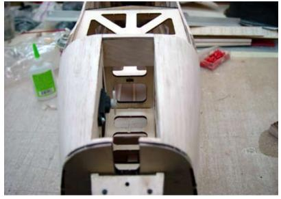
Fuselage forward bottom sheeting has been wet formed around the firewall and F2. The area between the sheets on F2 and the firewall are filled with 1/8" scrap.
