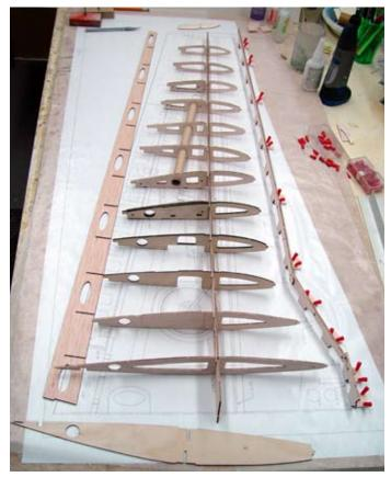
Above, the wing leading edge is in position and fastened to the bench. All ribs except the root and tip are in there appropriate slots in SW-B and on the left is SW-T which will be installed next. The outboard section of cable tunnel tubing must be installed prior to placing the ribs into the shear web slots. Once SW-T is installed, the ribs are captive in the sheer web assembly.
