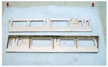
Above, the ailerons are being assembled over a piece of parchment paper. One aileron has been completed on one side and will now be turned over and completed. Note the 1/16" ply horn plate installed into the core sheet at the top of the photo.
