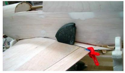
Above, FIL-A has been attached with a slurry of Epoxy and micro balloons. The lead weight and clamp assure that the fillet will conform closely to the wing.
