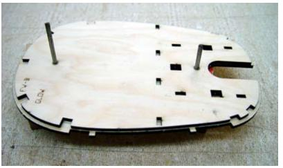
The firewall is being assembled from two 1/8" plywood sections. Epoxy and pin registration are used. Note that this is the glow firewall and is cut from aircraft ply while the electric firewall is cut from two sections of lite ply.
