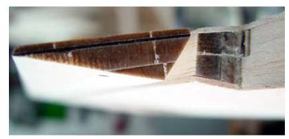
The flap assembly shown temporarily mounted to the wing. Cutting the shape on a band saw is quick and easy but must be done accuratly.
