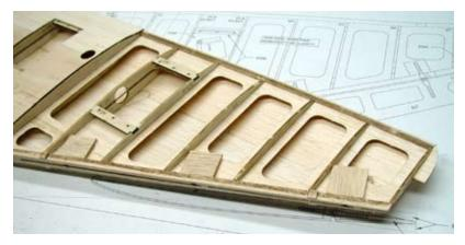
Partially assembled stabilizer section with only the bottom sheeting remaining to be added. All components are clearly visible here. Note the servo mounting screw rails between S2-BOT and S3-BOT, the hinge point caps, and leading and trailing edges.
