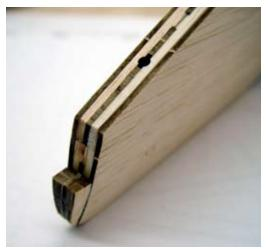
After sheeting, VT pieces are added and sanded to contour. Note the hinge pin openings are already provided and will assure a straight hinge line.
